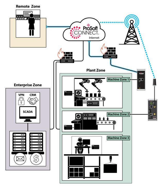
Each of these zones presents unique network security requirements and challenges. Understanding the challenges in each zone will help the enterprise network engineer determine the best solution that balances the production team's need for fast remote support, the safety manager's need to ensure personnel safety, and the enterprise network team's need to safeguard the company's data and information systems.
